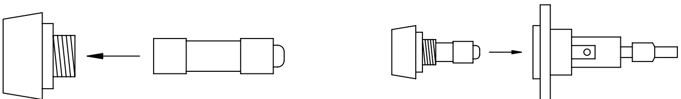
Figure 7. ORIENTATION OF FUSE IN HOLDER Fuse makes contact only when correctly installed. Place flat end of fuse in Cap. Place fuse & cap into fuseholder.
