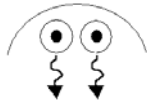
Figure 1: The reflectors are used to concentrate radiation down onto width up to 2.0 inches
