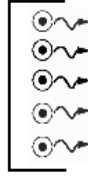
Figure 1: The reflectors are used to concentrate radiation down onto a 4.0-inch width.
